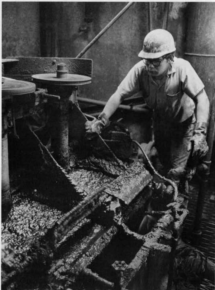
Flotation cell, a standard tool in mining for 50 years, here carries copper and molybdenum ore particles on bubble froth, while unwanted rock particles sink to cell bottom.
