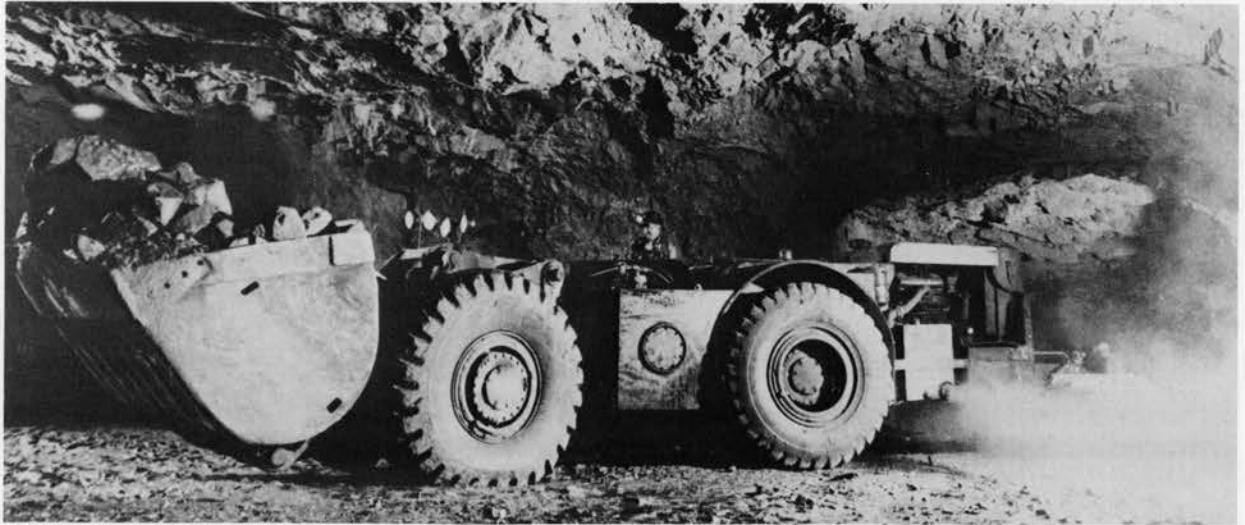
Advanced ore handling equipment includes diesel load-haul-dump vehicles such as this one that will pick up several tons of ore in one scoop.
